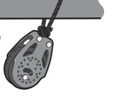
Using the other 520mm strop from the pack, attach a 40mm block to the new rear eye (which you added in step g).
