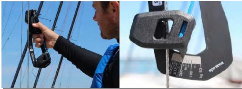
**Rig Tension:** Using a *Loos PT-1M* (Fig.1) on the forestay a **23** reading is a good general setting
