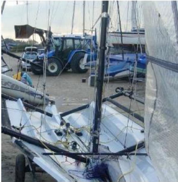
Figure 5: 27.7% of lowers height from jib track (old caps were longer)
