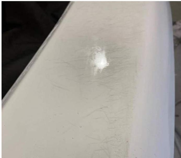
This issue can cheaply and easily be resolved by the application of thin rubber Heat shrink grip. This material is readily available from ebay and is available in various sized to suite the diameter of your tiller extension and in a range of colours. Simply slide the material over then extension and with a heat gun warm it and it will shrink tightly over for a permanent fit.
