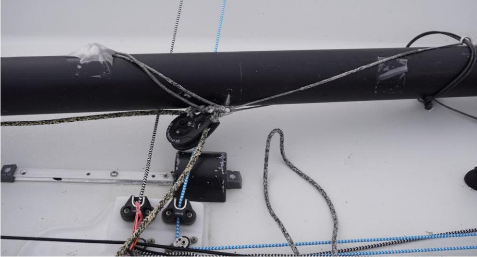
6 Move ratchet on boom forward 25cm by lacing between forward mainsheet eye and kicker eye
