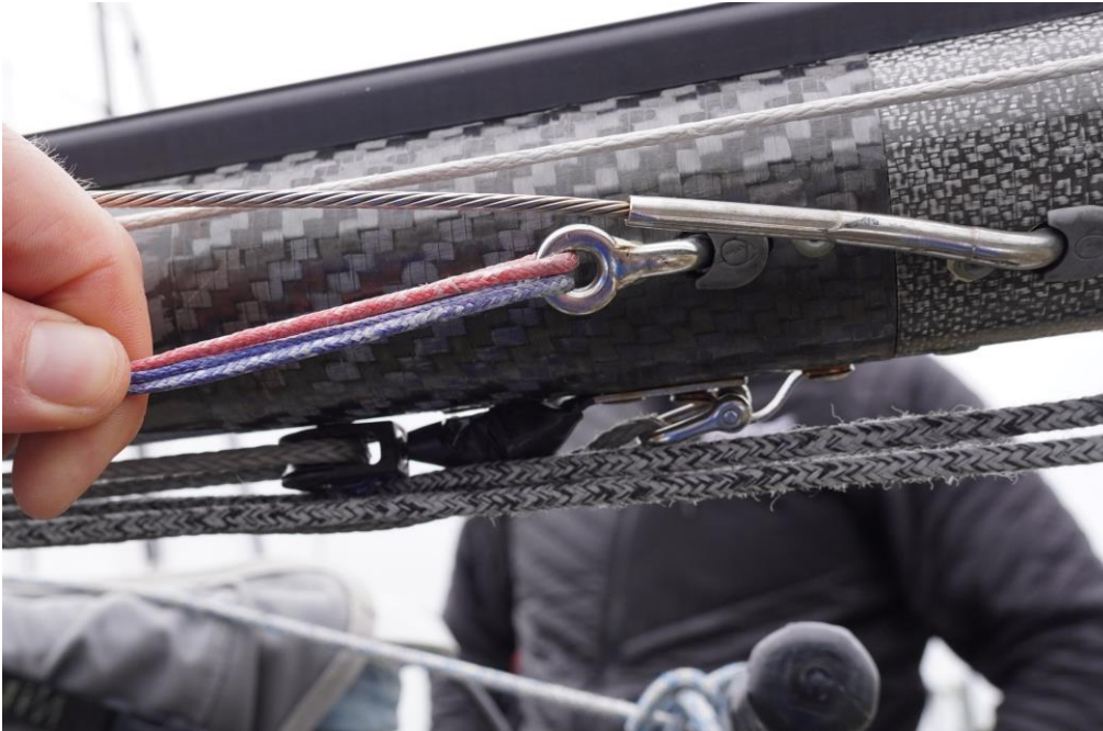
1 If going for 1.8m kiteline, ensure T terminal is well rounded and protect dyneema with outer covering. Check regularly. Alternatively, up to 2.5mm SK78 Dyneema
