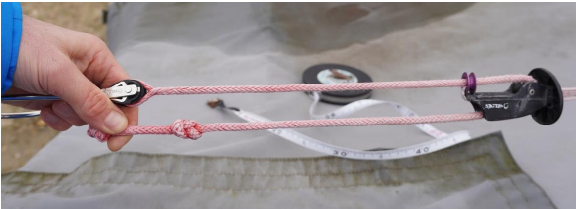
4 1:1 Trapeze adjuster. 4mm dyneema taken back inside itself. This is 75cm long including knots. It gives about 60cm of adjustment.
