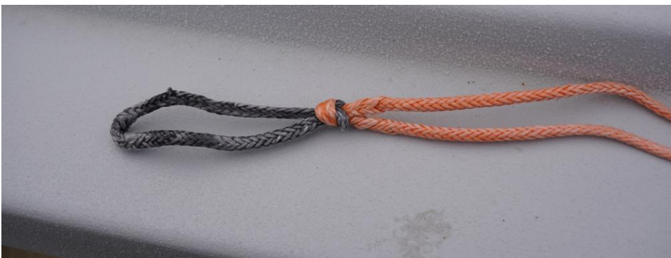
5 Kites sheets are tapered down to dyneema core and then eye spliced on to a dyneema loop which is used to clove hitch / luggage tag on to the spinnaker clew.
