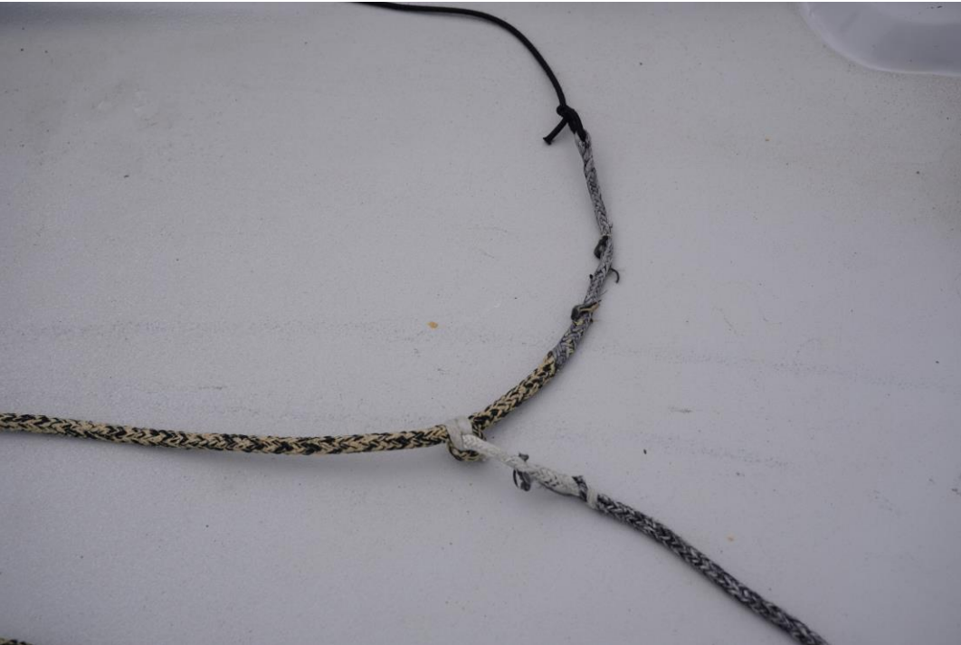
7 Mainsheet has small taper and spliced eye which take up elastic ties to. Jib sheet ties with a clove hitch on to a bite in the main. For take up elastic adjust length so tail of mainsheet is just within the gunwale with no stretch in take up elastic. Route elastic through central eye and to forward bend of bowsprit through offset hole in aft pole bung.
