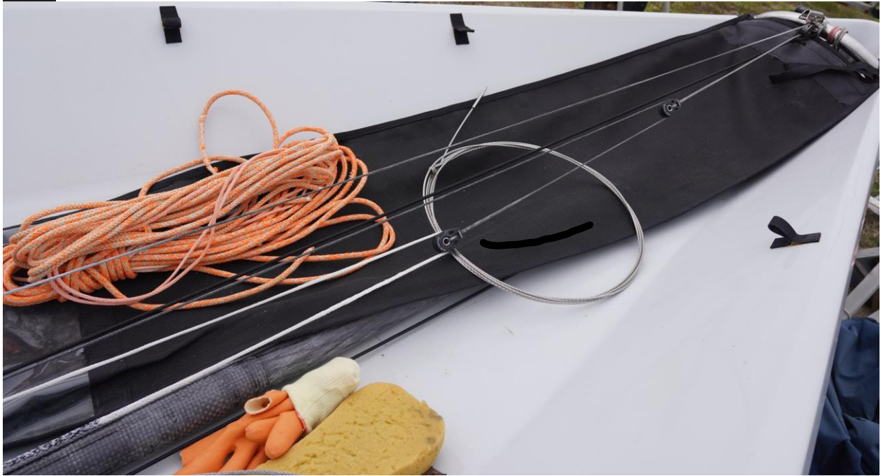
8 4:1 jib shown. This is a 2x2 cascade. This can be achieved by moving the block which is attached to the mast step to form half of the cascade.
