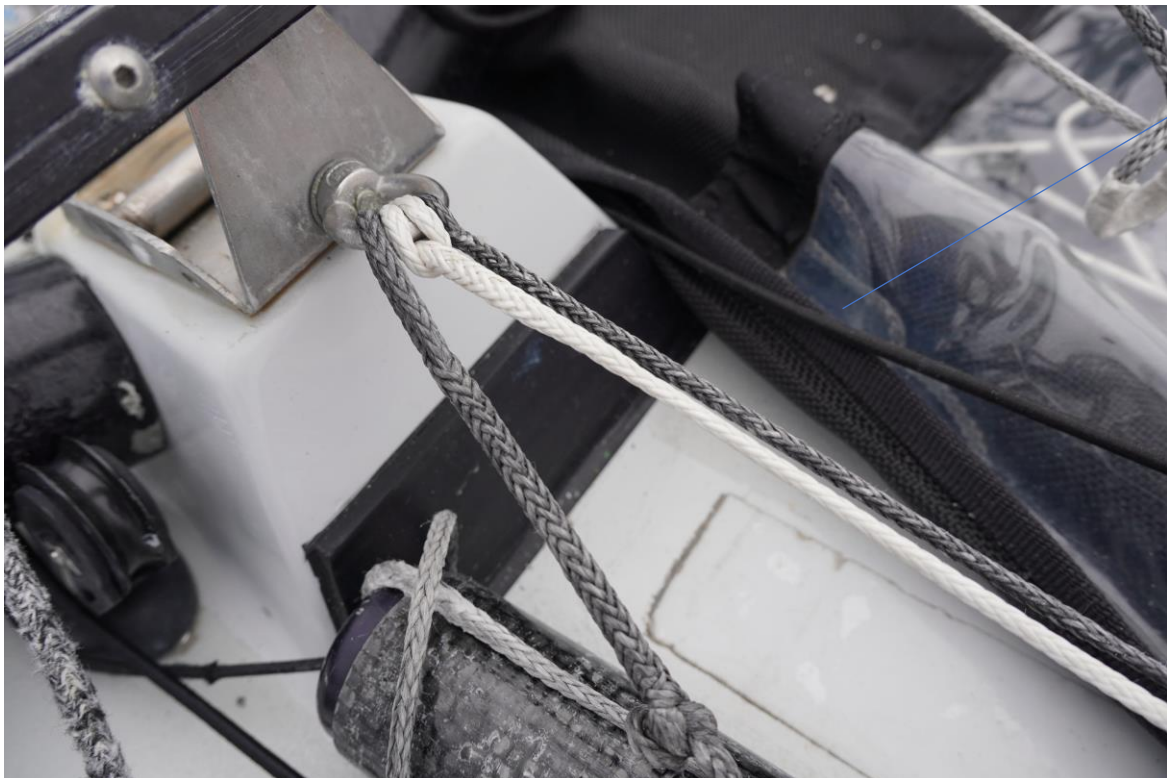
8 4:1 jib shown. This is a 2x2 cascade. This can be achieved by moving the block which is attached to the mast step to form half of the cascade.
