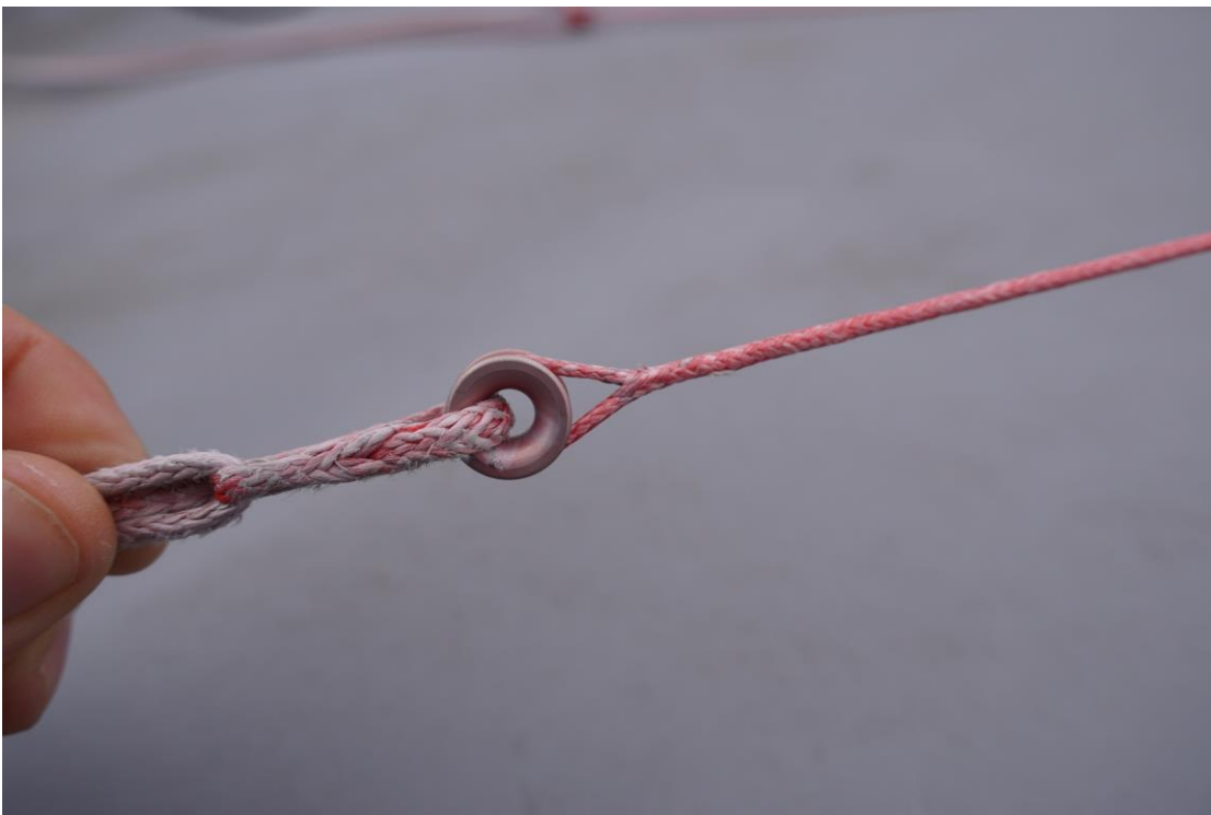
2 The length for the main trapeze line goes down to this low friction ring. Below this is a handle height adjuster which can be altered between 50 and 75cm.
